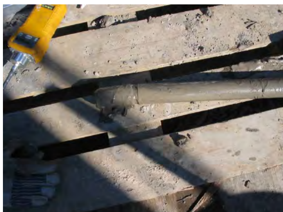
Photo 11: PID used to screen split-spoon samplers.
